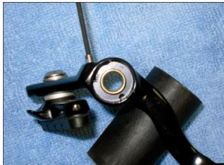
Tension Adjuster Plate – Correct Position
