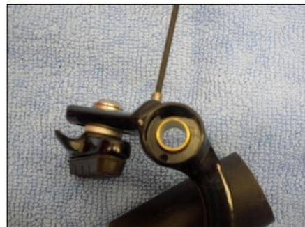
Tension Adjuster Plate – Blocking Adjuster Screw
