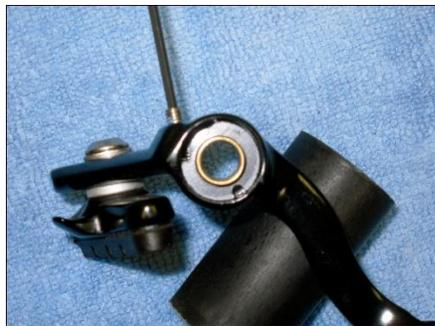
Tension Adjuster Plate – Correct Position
