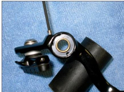
Tension Adjuster Plate – Correct Position
