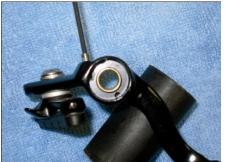
Tension Adjuster Plate - Correct Position
