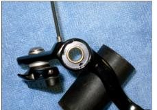
Tension Adjuster Plate – Correct Position
