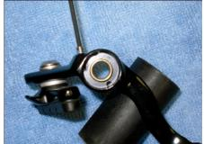
Tension Adjuster Plate - Correct Position
