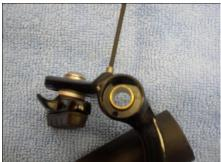
Tension Adjuster Plate - Blocking Adjuster Screw
