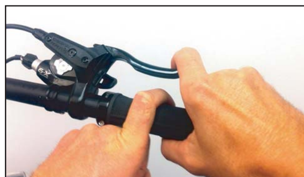
Brake lever should not contact finger after oil fill procedure.
