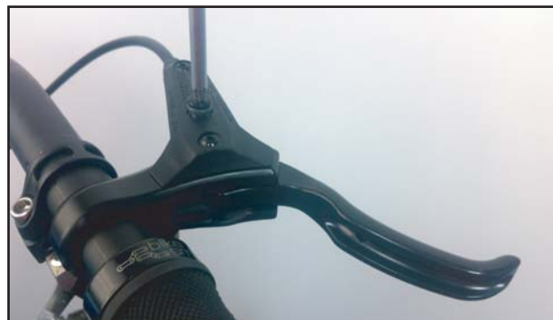
Position the lever horizontal - parallel with the ground.
