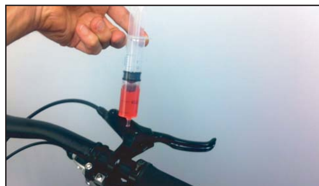
Add oil 5-6 drops at a time, pump lever and top off with oil.
