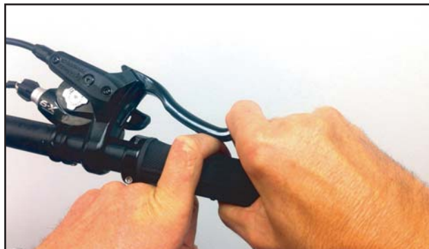
The 'finger test' method of checking oil fill in the brake
